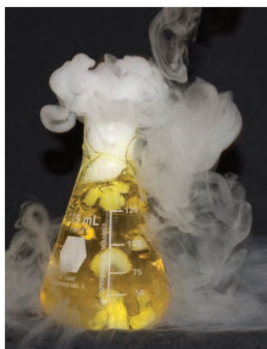
▲ When carbon dioxide sublimates, the gaseous \text{CO}_2 is cold enough to cause water vapor in the air to condense, forming fog.
