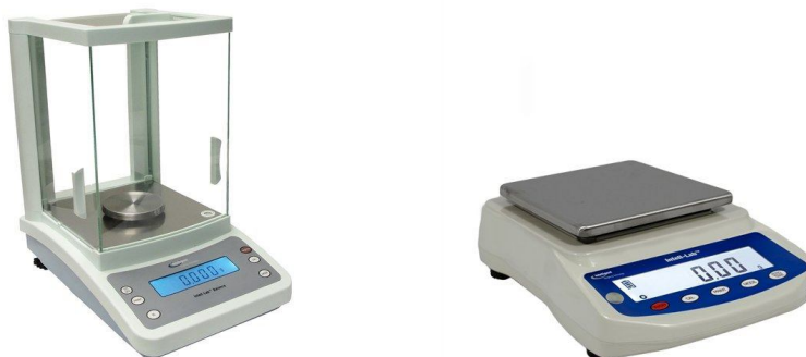
Figure 2. An analytical scale (left) and a centigram scale (right)
