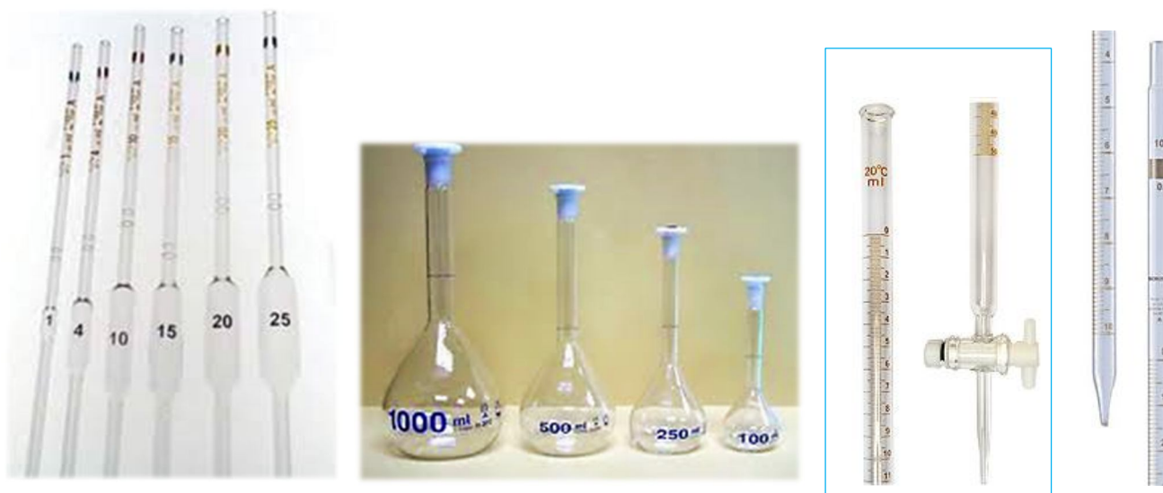
Figure 1. From left to right, volumetric pipets, volumetric flasks, a 50-mL buret (graduated), 10-mL Mohr pipet (graduated)
